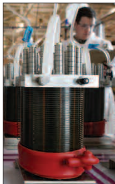
Proton PEM Electrolysis Stacks, the heart of HOGEN Generators
