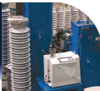
Photo: Leak test of surge arresters. By courtesy of ABB Inc., Youngwood, PA (USA).
